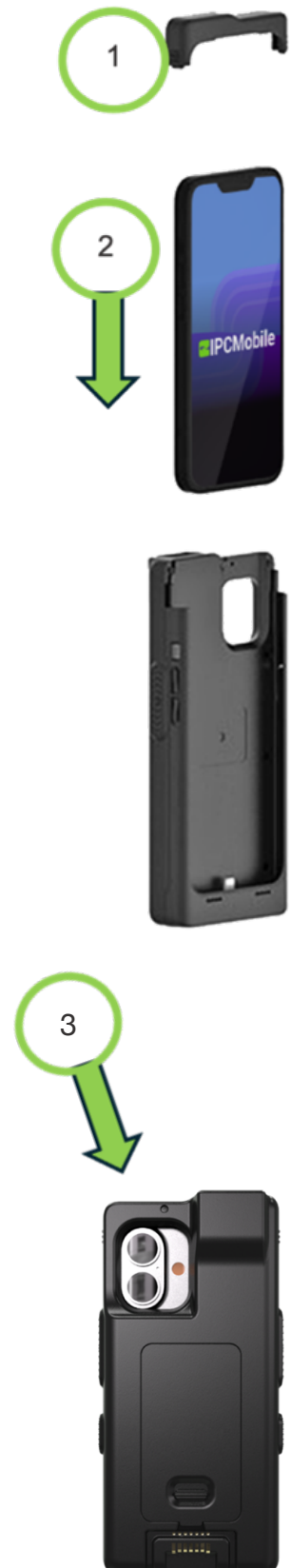
FIGURE 1: Installing an iPhone with the LPR
