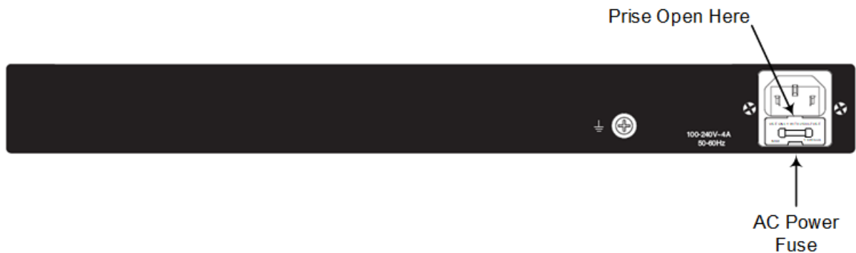
Figure 47: Opening the Fuse Cavity
