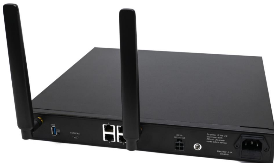
Figure 18: Connecting Cellular Antennas
