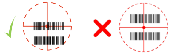
FIGURE 3: Illumination Box Showing Proper Barcode Reading / Aiming
